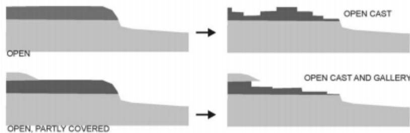
Figure 14 Examples of layered deposit geometries and the resulting quarry layout
