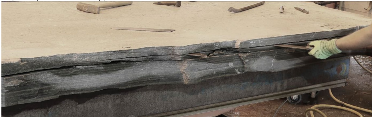
Splitting of slabs along the thin mica layers
