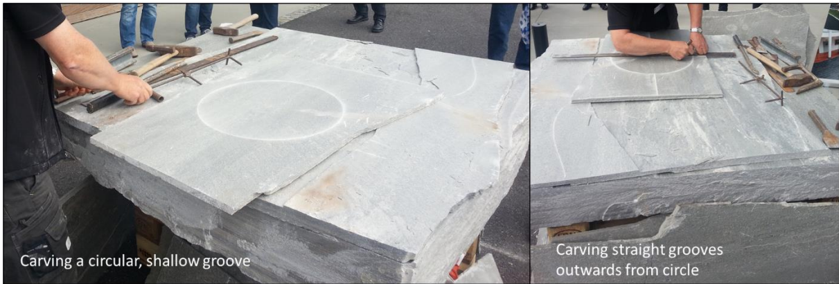
Figure 21. Carving shallow grooves for making a circular slab.
