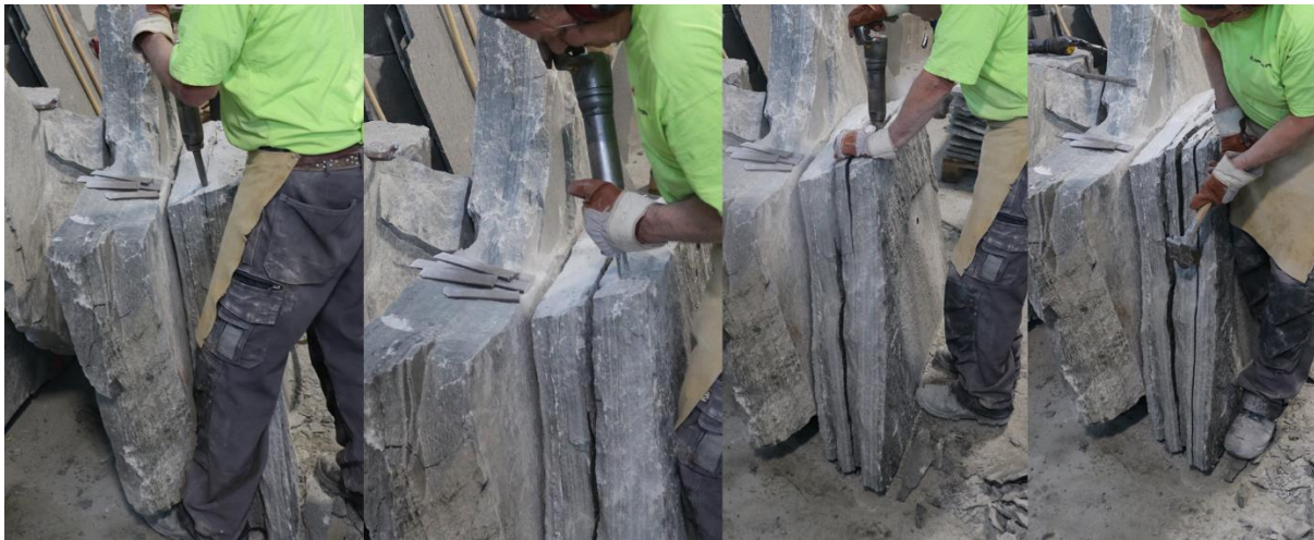
Figure 12. Using pneumatic wedge for splitting slabs. Note that the worker first split thick slabs, and then start splitting the thicker into thinner ones.
