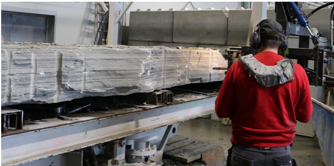
Figure 11. Aiming pneumatic wedge to impact mica layers.
