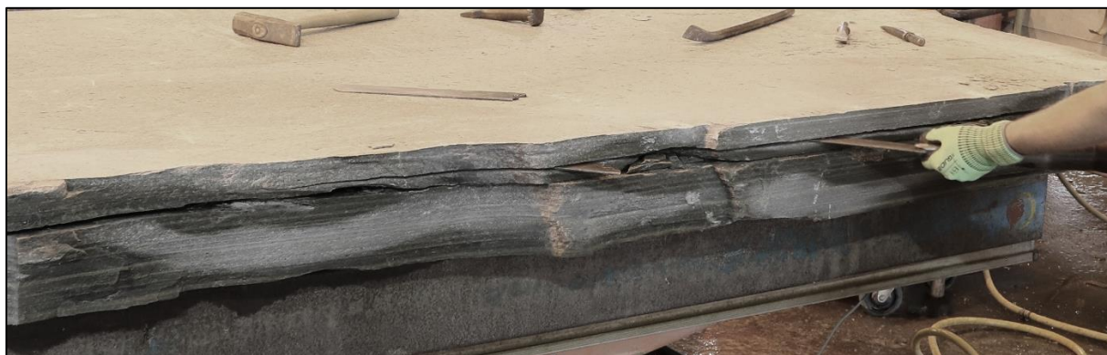
Figure 4. Splitting of slabs along the thin mica layers
