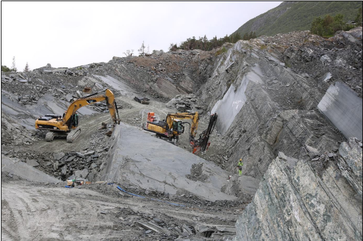
Figure 9. Diamond wire sawing employed for making cuts along the rift and hardway.
