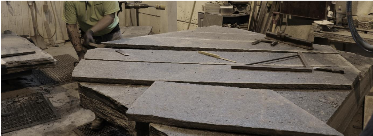
Figure 14. Breaking large slabs by levelling.
