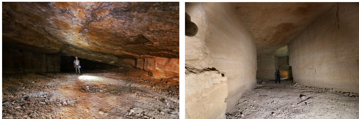
Fig. 17: Inside view of quarry landscape (cave) was developed during the exploitation of calcarenite for the production of building stone. The left one shows the landscape of a cave in Acropolis in the premises of the Headquarters of the Cyprus Telecommunications Authority (CYTA) and the right one is located in Mammari west of Nicosia.
