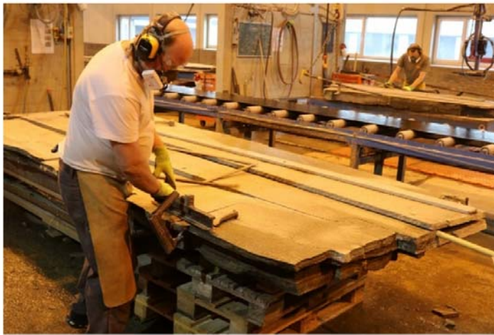
Traditional breaking of schist slabs, Oppdal, Norway
