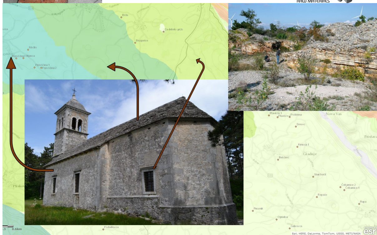
Figure 6. Provenance analysis of limestone made architectonic elements linked each limestone type with the mapped geological unit and, where possible, with its source quarry. Reproduced from Novak (2015).
